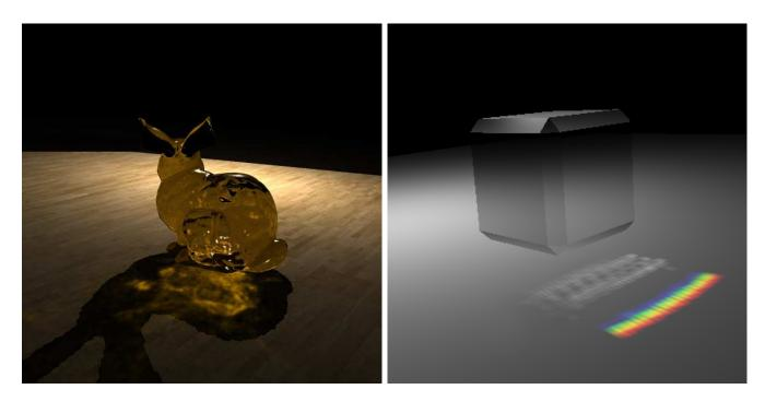
Fig. 9. (Left) Colored caustics from a refractive bunny with light attenuation in different color channels. (Right) Diffraction grating effect obtained using the caustic mapping algorithm with different refractive indices for each of the three RGB color channels.
