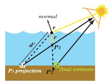
Fig. 4. Diagram of the intersection estimation algorithm. The solid-lined arrows correspond to the position texture lookups.
