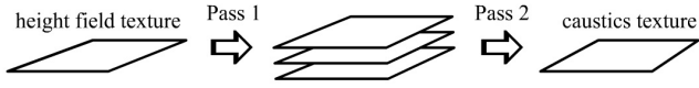
Fig. 4 The two-pass algorithm: the first pass reads the height field texture and generates multiple outputs; the second pass reads the result of the first pass and produces the final caustics map.
