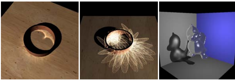
Figure 1: A real-time rendering of a metal ring and its caustics on a wood plate at more than 95 frames per second. A subset of the glossy pixel lights is shown in the center image. A refractive glass tweety (only refraction at the back-facing surface) runs at 150 frames per second.
