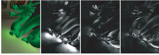
Figure 5: Temporal coherence between two successive animation frames. From left to right: the brightened indirect illumination, frame-to-frame difference using RSMs with 256 VPLs, difference using image-space radiosity, and difference using hierarchical image-space radiosity.
