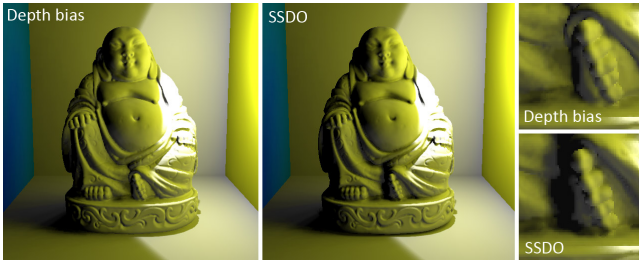
Figure 11: Instant Radiosity with screen-space shadow correction. Shadows of small details, like the toes, are lost due to the depth bias. These small shadows can be restored in image space.
