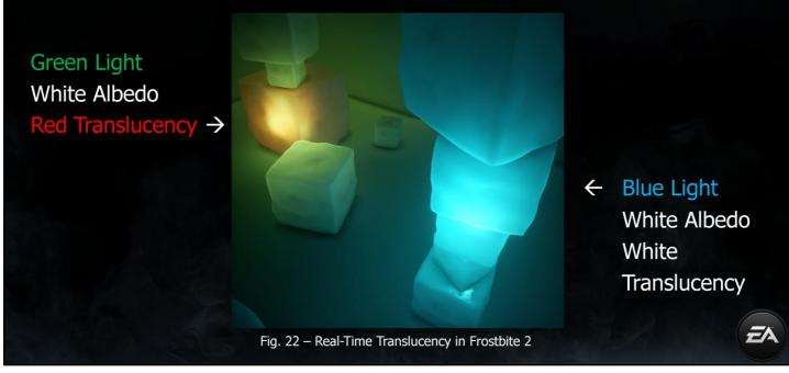
Here's a result with colored translucency. The cube on the left has a red local thickness texture, but the light inside its convex hull is green, in comparison to the object on the right, where the local thickness texture is greyscale.
